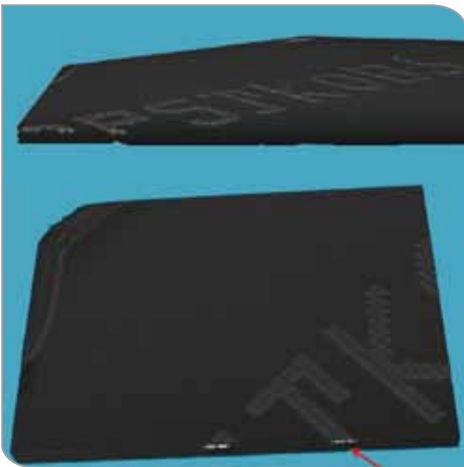
Figure 3: 3D-XRDI image of a wafer laser mark. The red arrow points to the strain fields created by the laser mark process.
