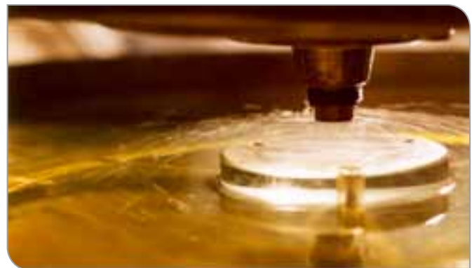
Figure 1: UO 2 droplets forming during sol-gel process
