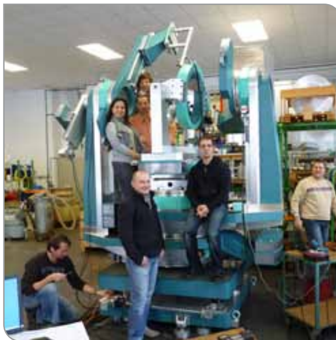
Figure 1: Installation of the new diffractometer for the NANO beamline
