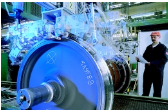
AURA - Automated ultrasonic railroad wheel set inspection system
