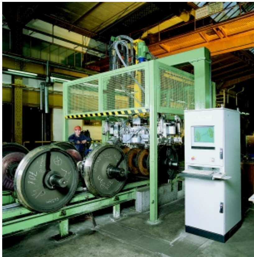
Figure 1: Wheel set testing station »AURA« at the Nürnberg maintenance facility (Deutsche Bahn)
