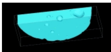
Figure 4: 3D-CT Volumetric section of a concrete sample
