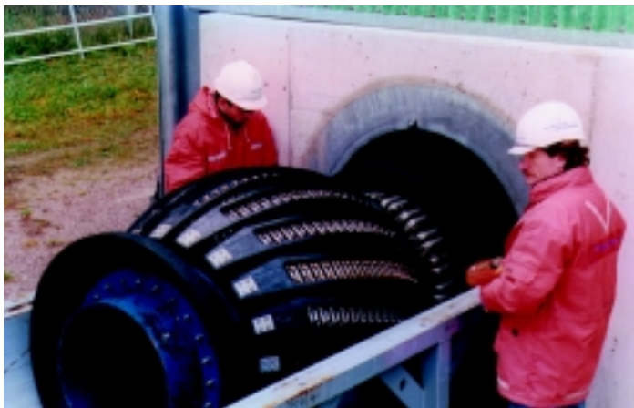
EMUS-Testing of pipelines
