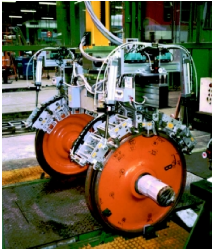
Figure 2: Wheel set testing station »AURA« at the Munich maintenance facility (Deutsche Bahn)
