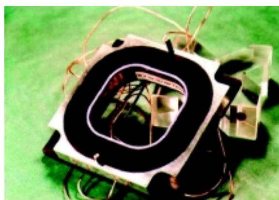
Figure 4: 400-channel ring array; the light-colored inside ring contains the piezo-electric transducers, the dark ring covers the cabling
